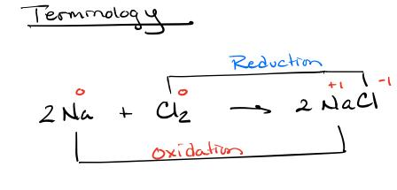
Species being oxidized Na metal Species being reduced Clz gas Oxidizing Agent (reagent) Clz gas The species causing the sodium to be oxidized Redusing Agent (reagent) Na metal The species causing the Clz to be reduced
